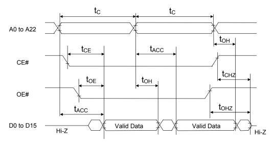
8-BIT READ MODE (BYTE $\# = V_{IL}$ )
