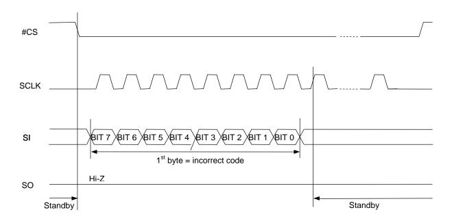
Incorrect command makes this LSI become and keep standby mode until next #CS rising edge. In standby mode, SO pin is High-Z.
