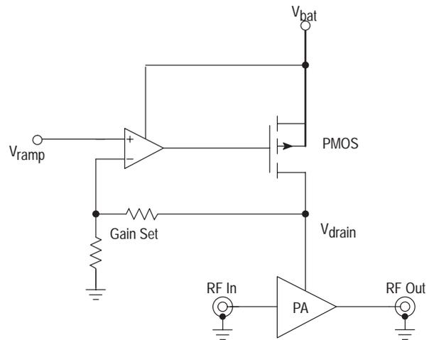
**NOTE:** The positive voltage generated by the Buffer stage can be used to supply the OpAmp and make it possible to drive a NMOS switch as a voltage follower. Doing so, the main advantage is to have a lower R<sub>dson</sub> switch and better intrinsic linearity.
