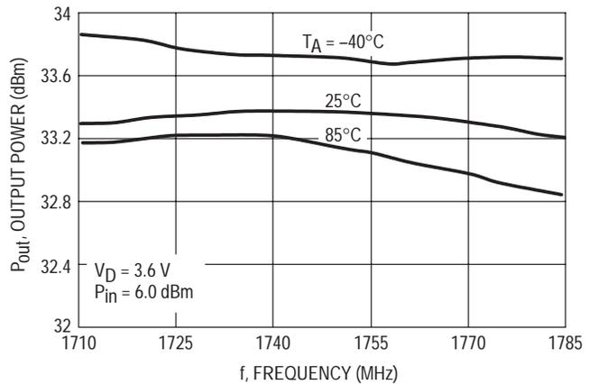
Figure 8. Output Power versus Frequency
