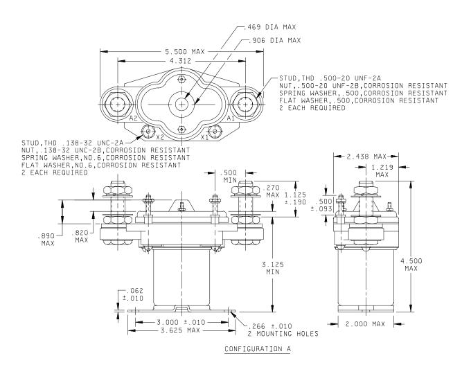
FIGURE 1. <u>Dimensions and configurations</u>.
