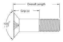
Use the MS24694 series to replace AN509 screws of like material and finish. SEE THE CHARTS for desired size numbers. SEE CROSS REFERENCE on next page for Superseding Part Numbers.
