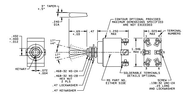
FIGURE1. <u>Dimensions and configuration</u>
