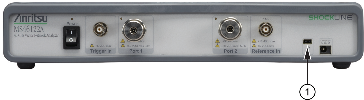
Figure 2-4. ShockLine MS46122A Series VNA USB Connection
