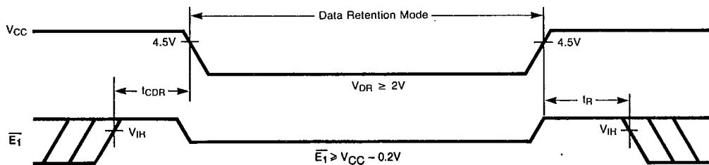
LOW  $V_{CC}$  DATA RETENTION WAVEFORM (2) ( $E_2$  Controlled)
