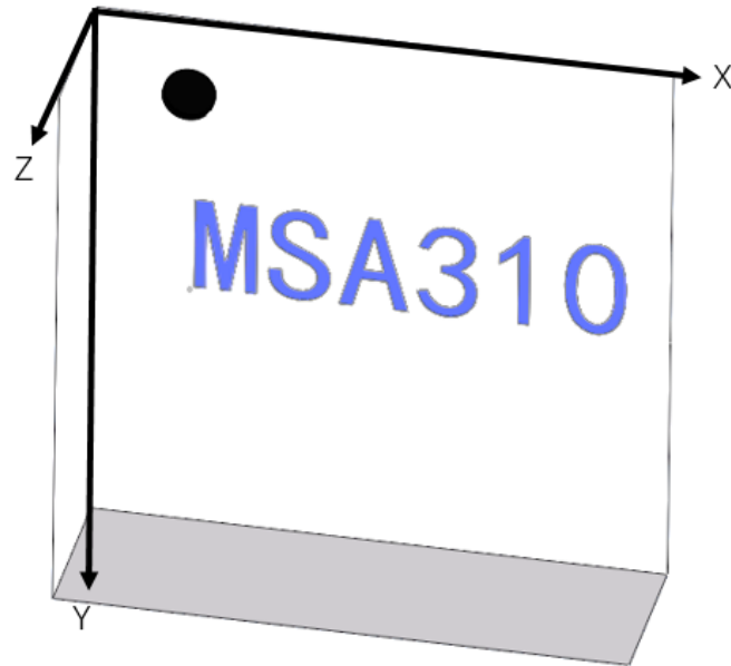
Figure 10: Orientation of sensing axis
