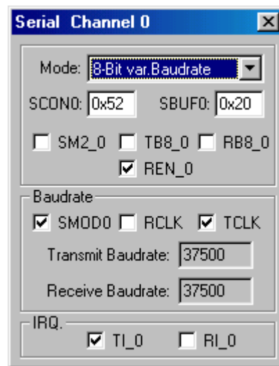
Figure 17-19. Serial Channel 0 Communication Peripheral
