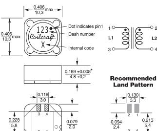
\* For optional tin-lead and tin-silver-copper terminations, dimensions are for the mounted part. Dimensions before mounting can be an additional 0.012 inch (0,3 mm)
