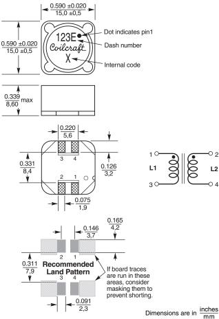
Excellent coupling coefficient ( $k \ge 0.98$ ) and 500 Vrms isolation makes the MSD1583 series of coupled inductors ideal for use in a variety of circuits including flyback, multi-output buck, SEPIC and Zeta. These parts provide high inductance, high efficiency and excellent current handling. In SEPIC topologies, the required inductance for each winding is half the value needed for two separate inductors, allowing selection of a part with lower DCR and higher current handling.
