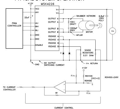
This is a diagram of a typical application of the MSK4226. The design VCC voltage is +12 volts and should have a good low ESR bypass capacitor such as a tantalum electrolytic. The digital inputs can come from a microprocessor or any type of PWM controller. The controller will use the current sense signal to either control current through PWM, current limit the bridge, or both.
