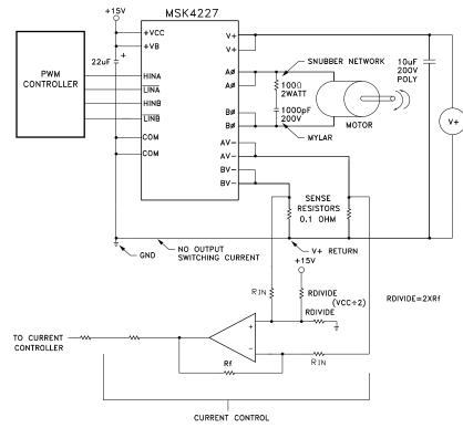
This is a diagram of a typical application of the MSK4227. The design + VCC voltage is + 15 volts and should have a good low ESR bypass capacitor such as a tantalum electrolytic. The digital inputs can come from a microprocessor or any type of PWM controller. The controller will use the current sense signal to either control current through PWM, current limit the bridge, or both.
