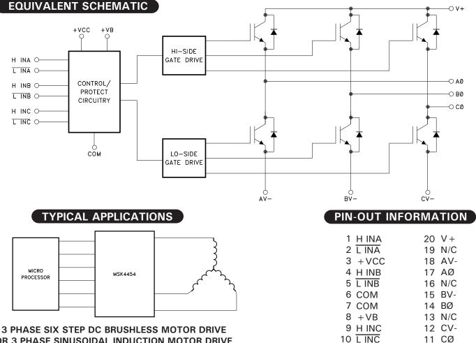
**OR 3 PHASE SINUSOIDAL INDUCTION MOTOR DRIVE**
