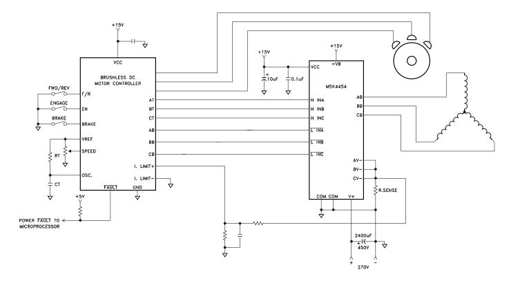
The MSK 4454 is designed to be used with a +270 volt high voltage bus, +15 volt low power bus and +5 volt logic signals. Proper derating should be applied when designing the MSK 4454 into a system. High frequency layout techniques with ground planes on a printed circuit board is the only method that should be used for circuit construction. This will prevent pulse jitter caused by excessive noise pickup on the current sense signal or the error amp signal.
