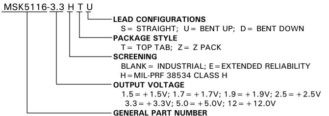
The above example is a +3.3V, Military regulator using the top tab package with leads bent up.
