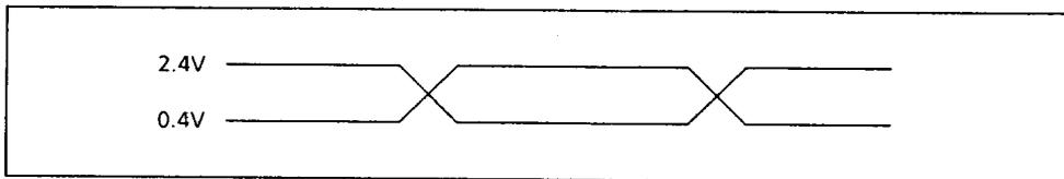
● **Voltage at AC Timing Measurement Point**
