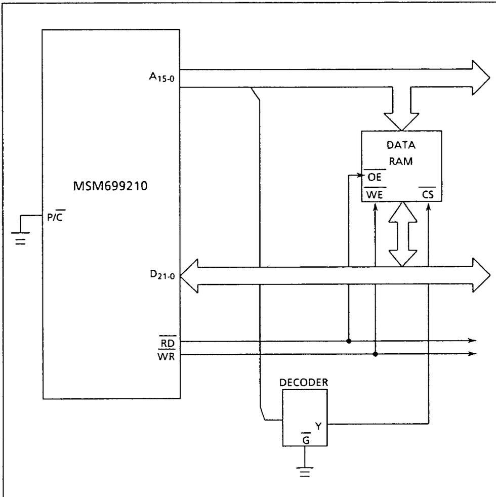
4.3 MPU Interface (Processor mode)
