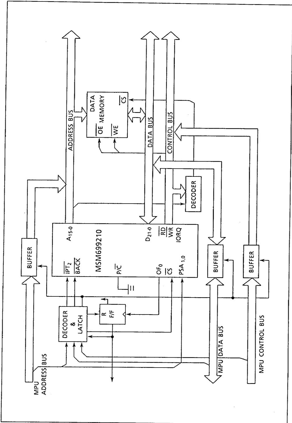
4.5 Multi-DSP Interface (Processor mode and controller mode)
