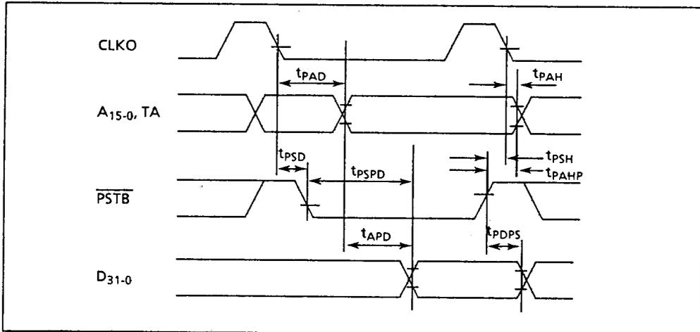
● External Data Write Timing (No wait cycle: processor mode & controller mode)
