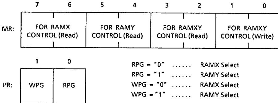
The 8-bit mode register is used to specify the RAMX and RAMY addressing mode. The RAMX, RAMY, and RAMXY addresses are determined by arithmetic operations executed on index registers (IXR, IYR, and IZR) and instruction offset (XA, YA, XYA, and ZA) in accordance with the contents of this mode register.
