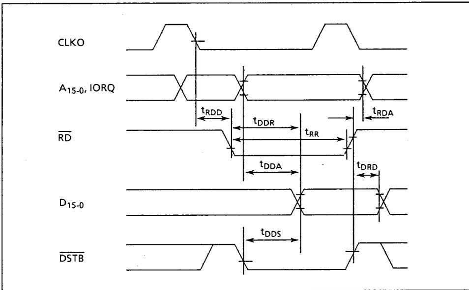
● External Data Access Timing (Some wait cycle: processor mode & controller mode)
