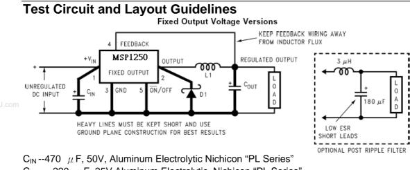
$C_{IN}$ --470  $\mu$  F, 50V, Aluminum Electrolytic Nichicon "PL Series"  $C_{OUT}$  --220  $\mu$  F, 25V Aluminum Electrolytic, Nichicon "PL Series" D<sub>1</sub>--5A, 40V Schottky Rectifier, 1N5825 L<sub>1</sub> --68  $\mu$  H, L38
