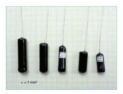
The Lotek Sensor Transmitter series has expanded to include tags of much smaller size than previously available enabling biologists to collect physiological data (temperature and motion status) on smaller adult and juvenile fish species. In addition, the MST-series incorporates advanced programming algorithms to facilitate extended operational life and variable bu rst rate to match project temporal resolution requirements
