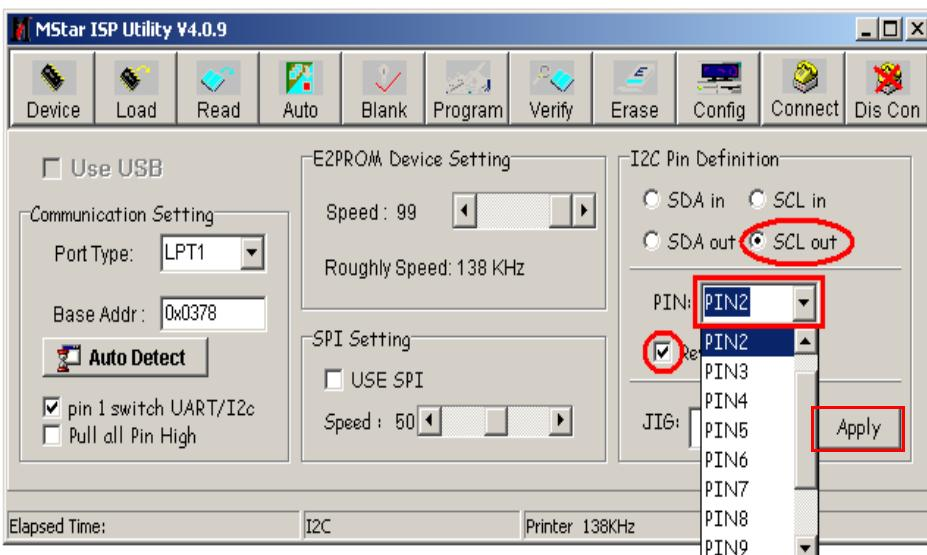
After having finished all above, clicking the "Apply" button to complete the configuration.
