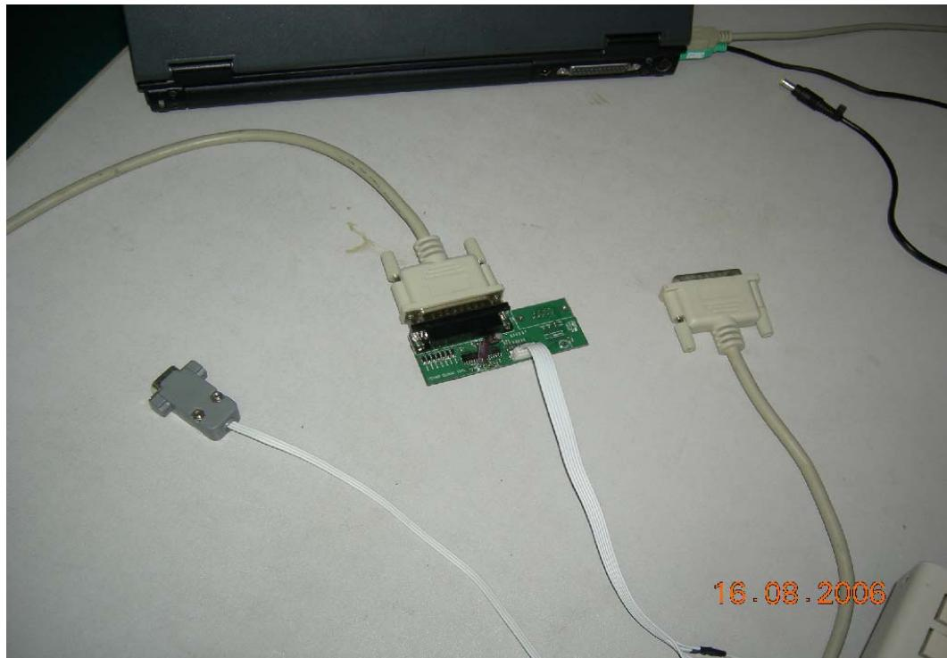
Connect the Debug board to the TV use VGA interface, the other parallel port to the computer, just as the following.
