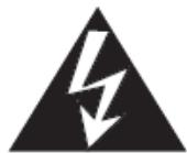
The lightning flash with arrowhead symbol, within an equilateral triangle is intended to alert the user to the presence of uninsulated dangerous voltage within the products enclosure that may be of sufficient magnitude to constitute a risk of electric shock.
