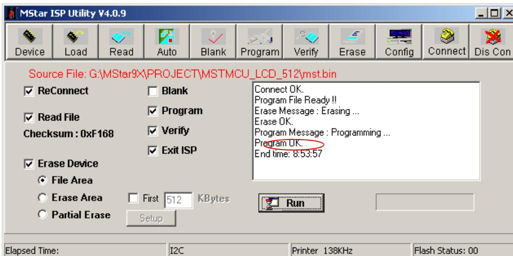
The above appears on the screen-the word “program ok” shows in the information displaying window, indicating upgrading is over.
