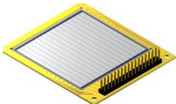
Design W1(DS)-300 2M on a standard FR4 transmission package*.
