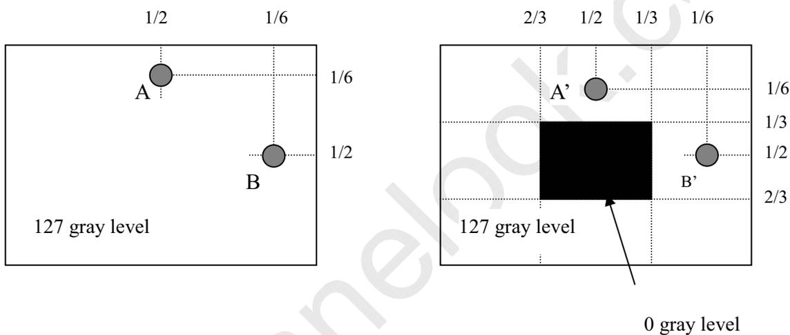
$|L_A - L_{A'}| / L_A \times 100\% = 2\% \text{ max.}$ ,  $L_A$  and  $L_{A'}$  are brightness at location A and A'
