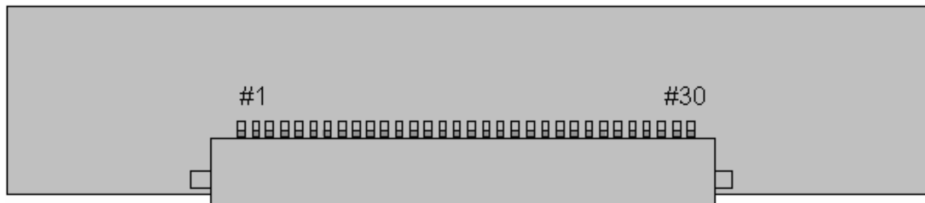
Top view of LVDS connector
