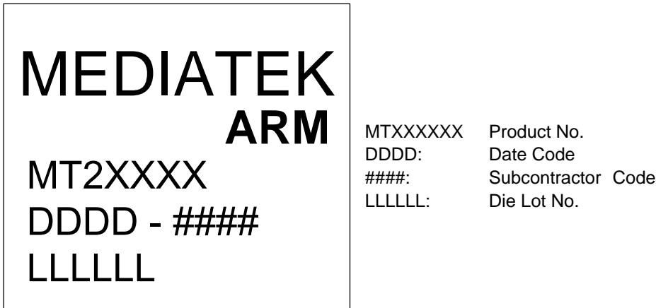
Figure 7. Mass production top marking of MT2502A
