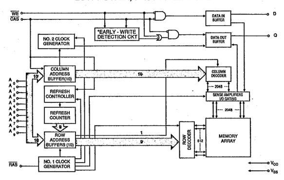
\*NOTE: WE LOW prior to CAS LOW, EW detection CKT output is a HIGH (EARLY WRITE) CAS LOW prior to WE LOW, EW detection CKT output is a LOW (LATE WRITE)
