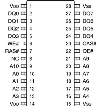
cycles. The address is entered first by RAS# latching 11 bits (A0-A10) and then CAS# latching 10 bits (A0-A9).
