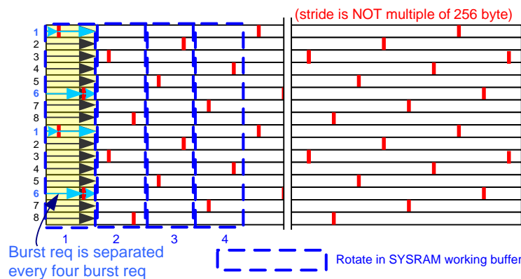
Figure 6-23. 4-16 burst in 270° rotation with/without flip
