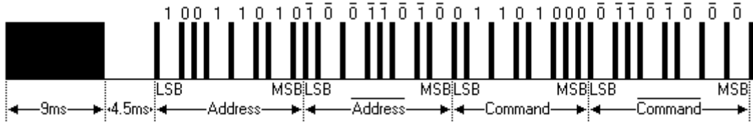
Figure 5-23. Pulse train in transmission of NEC protocol
