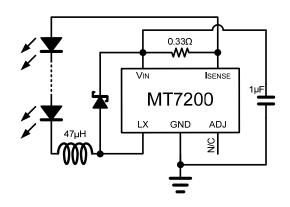
Output current can be adjusted above, or below the set value, by applying an external control signal to the 'ADJ' pin.
