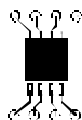
b) 105^\circ\text{C}/\text{W} when mounted on a .04\text{ in}^2 pad of 2 oz copper
