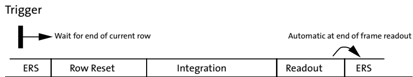
Figure 39: Entering and Leaving a Global Reset Sequence
