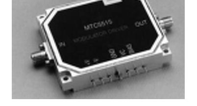
The MTC5515 is a precision GaAs medium power amplifier. It operates from 30 KHz to 11 GHz and exhibits a flat linear gain response. The MTC5515 has low internal jitter making it useful for digital applications. The self-contained module operates from a +8V and a -5V power supply. It is fully hermetic, consumes 5 W of power and operates over a case temperature range from 0°C to +70°C.
