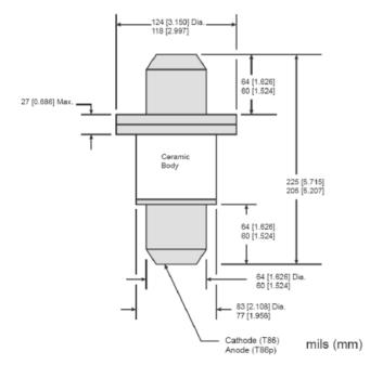
Package Capacitance (C\_\_\_\_) = 0.17 pF
