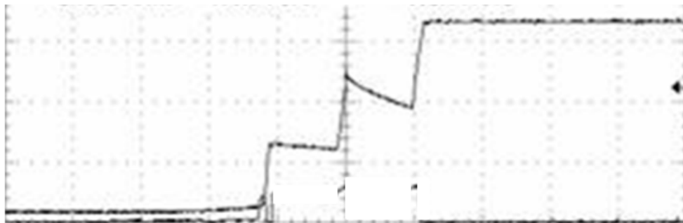
Figure 22. Supply Voltage Drop
