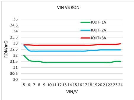
Internal on resistance vs input voltage
