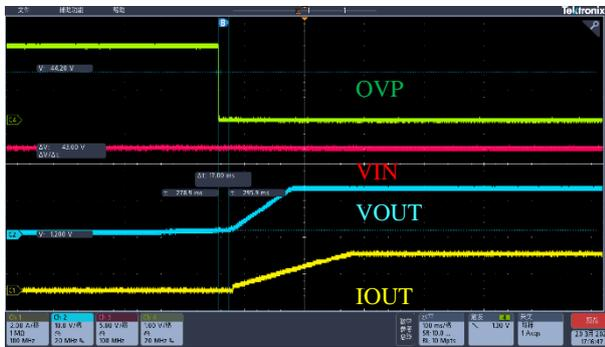
Input over voltage protection release
