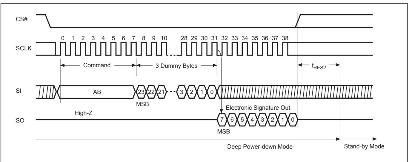
**Figure 29. Release from Deep Power-down (RDP) Sequence (Command AB)**
