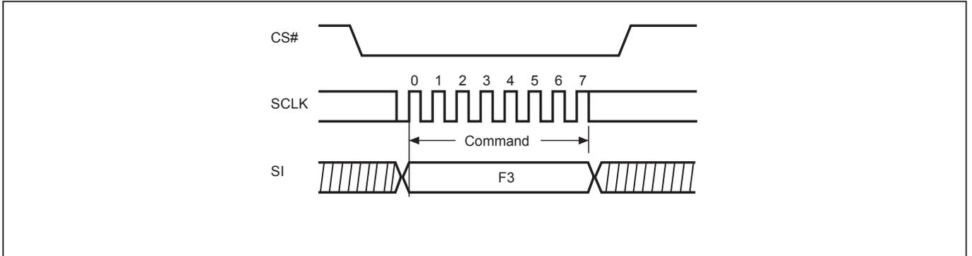
**Figure 15. Read Data Bytes (READ) Sequence (Command 03)**
