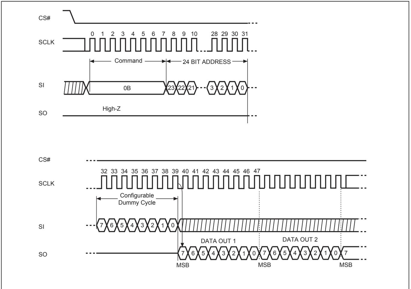
Figure 18. 2 x I/O Read Mode Sequence (Command BB)
