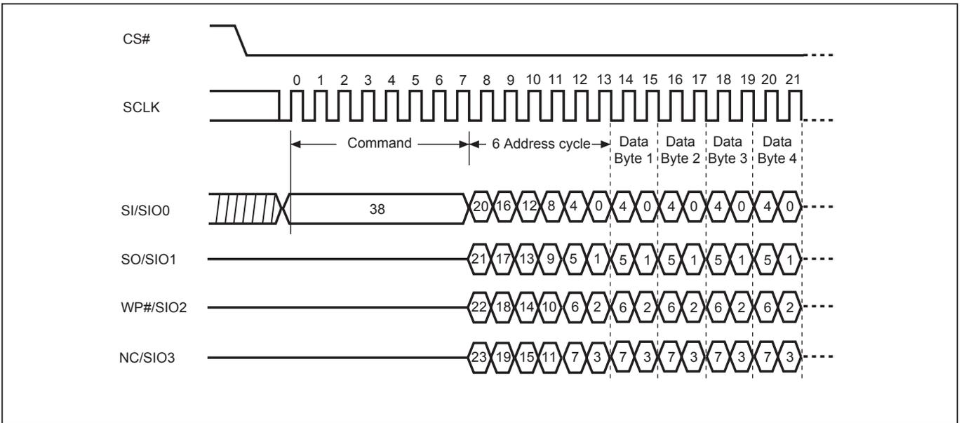
**Figure 23. Continuously Program (CP) Mode Sequence with Hardware Detection (Command AD)**
