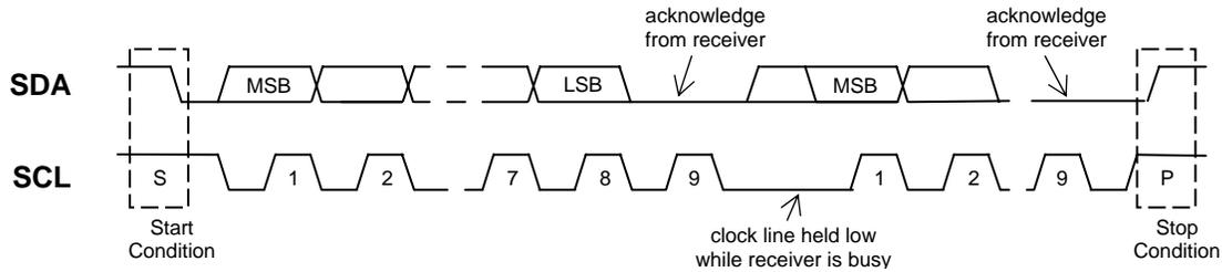
The MX3000CS I<sup>2</sup>C commands are always sent in three adjacent bytes – address, mode and data as shown in Figure 7.
