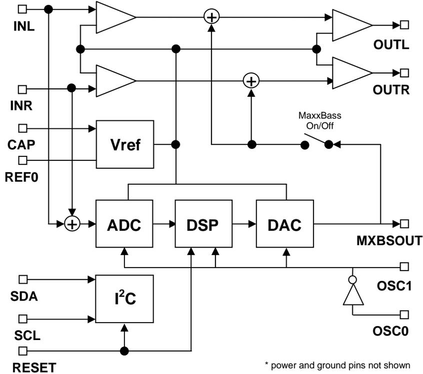
All internal clocks are established from a crystal oscillator, ceramic resonator or other clock source. The relationship between the clock frequency input, sigma delta ADC/DAC converter clock, DSP sample rate and MaxxBass Frequency is shown in Figure 2.
