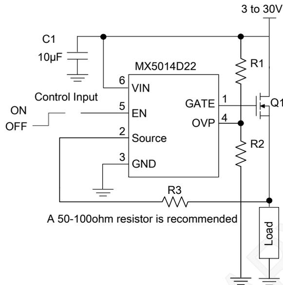
Typical application with high side NMOSFET driver
