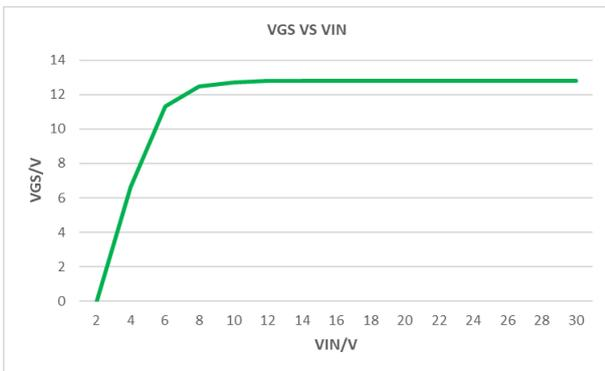
Vgate – Vsource vs Input voltage
