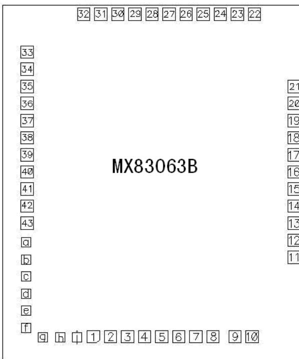
Substrate Size: 2400 μm × 2700 μm
