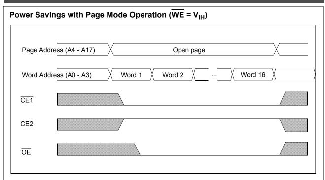
Note: Page mode operation is a method of addressing the SRAM to save operating current. The internal organization of the SRAM is optimized to allow this unique operating mode to be used as a valuable power saving feature.
