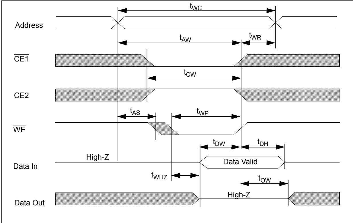
**Timing Waveform of Write Cycle ( $\overline{CE1}$  Control)**
