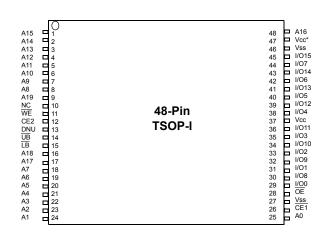
Note: Pin#47 on the TSOP-I Package must be tied to Vcc.
