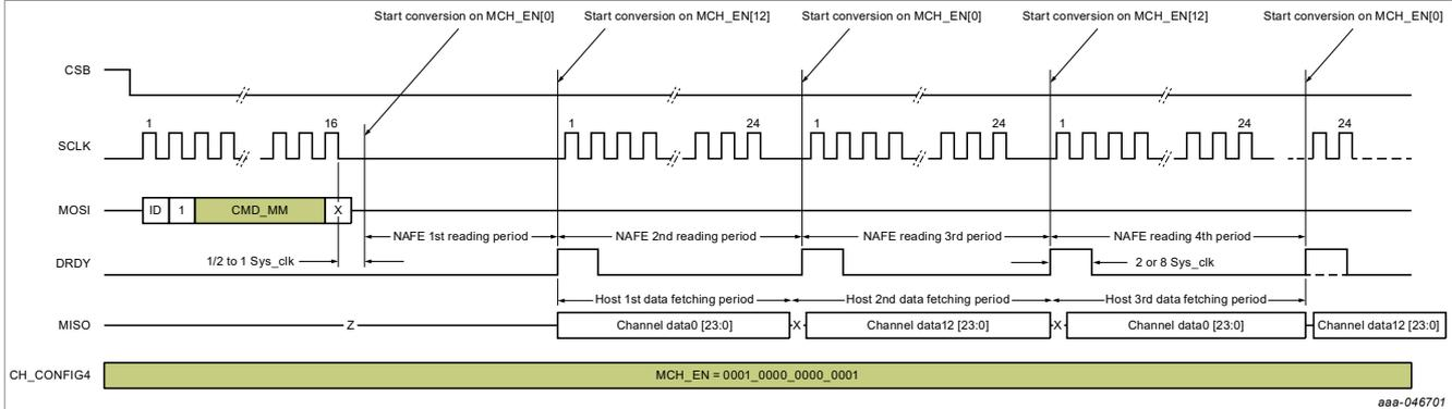
Figure 26. Timing diagram - MCCR
