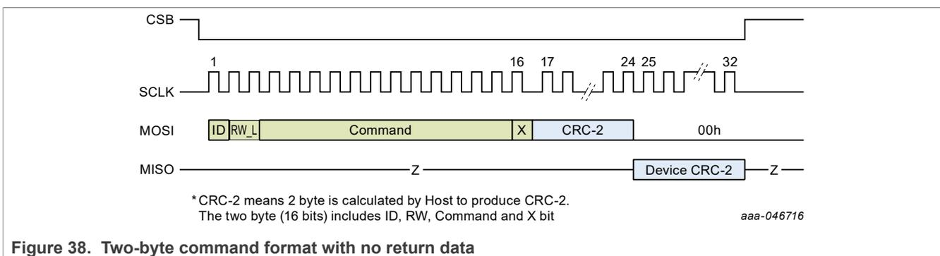
Figure 38. Two-byte command format with no return data
