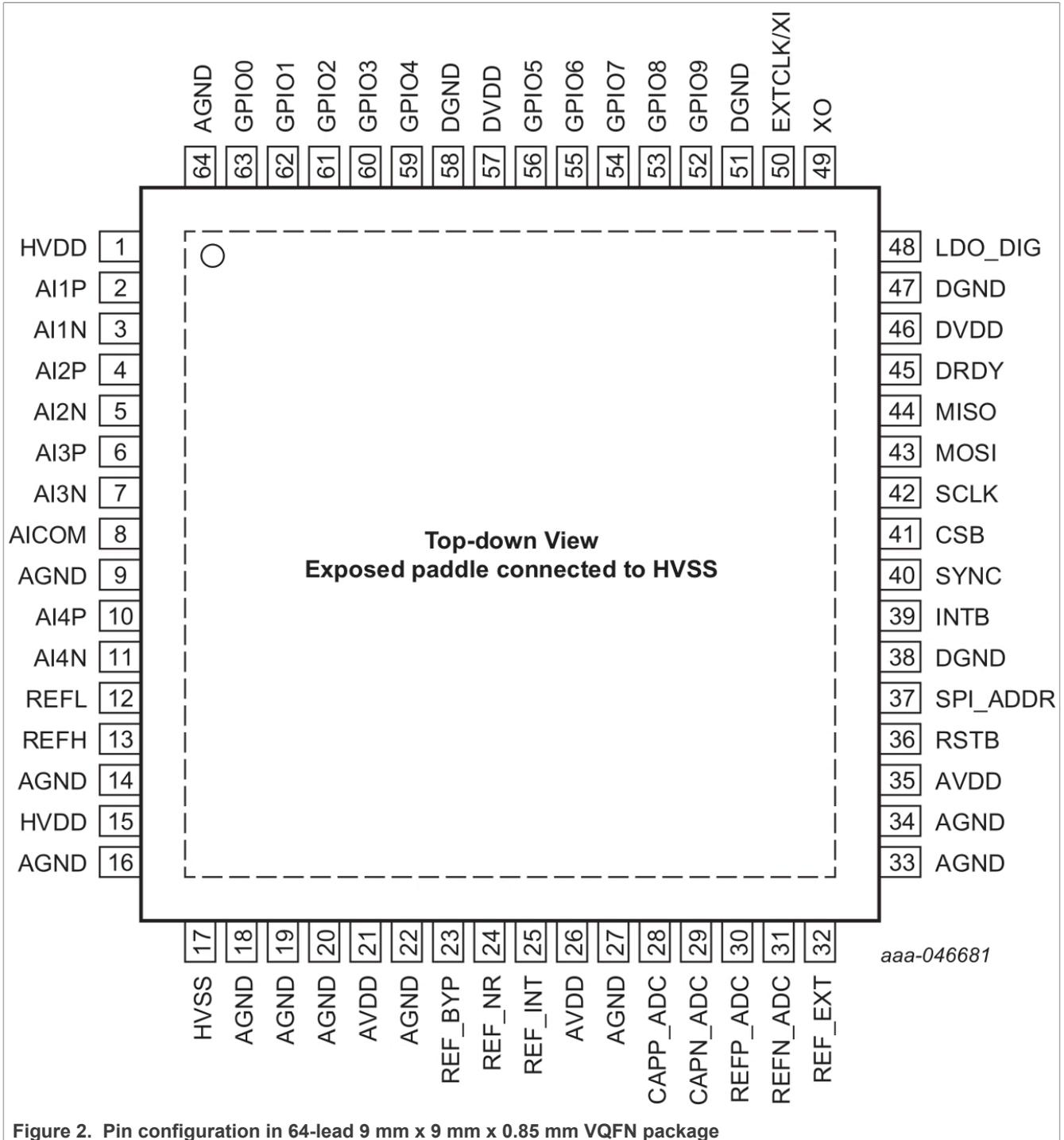
Figure 2. Pin configuration in 64-lead 9 mm x 9 mm x 0.85 mm VQFN package
