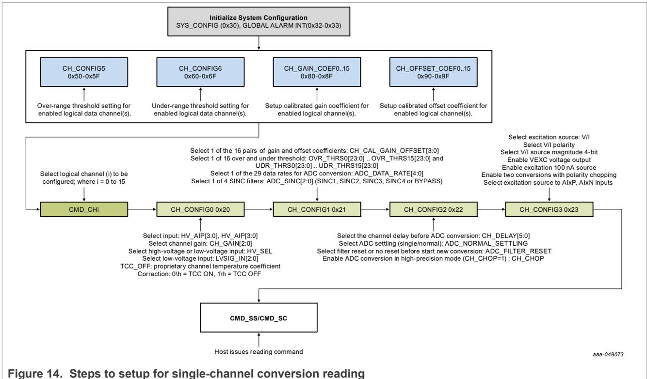
Figure 14. Steps to setup for single-channel conversion reading
