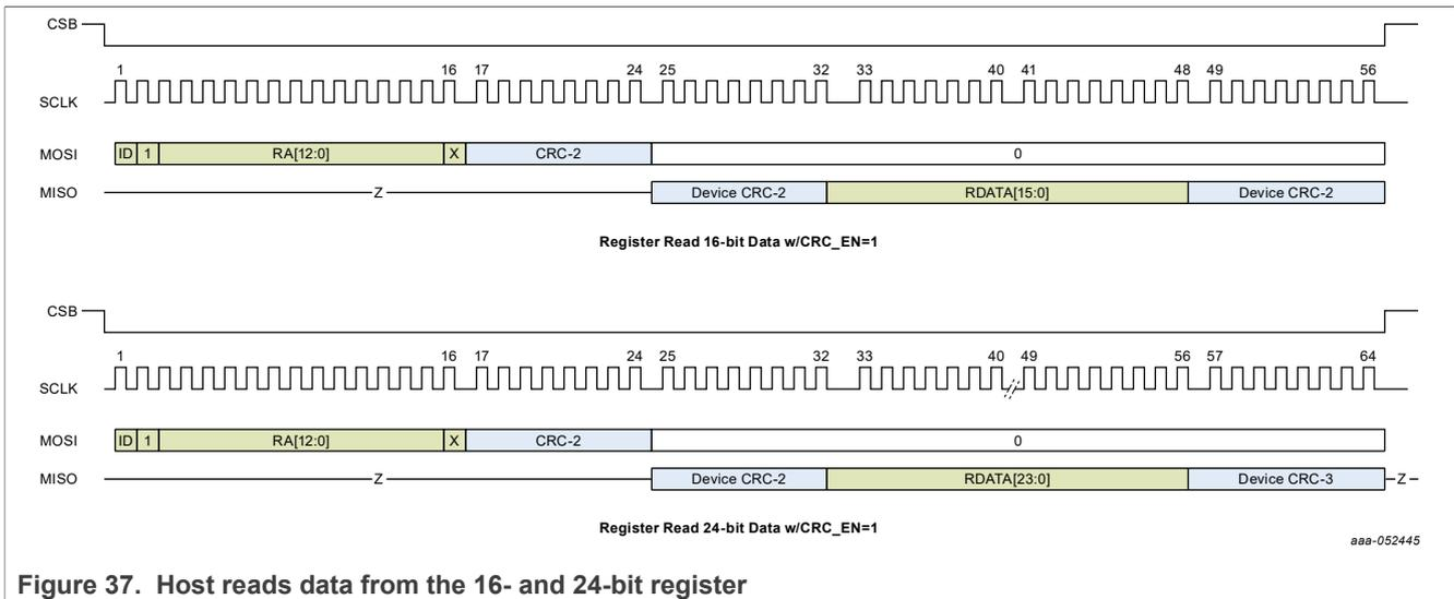
Figure 37. Host reads data from the 16- and 24-bit register
