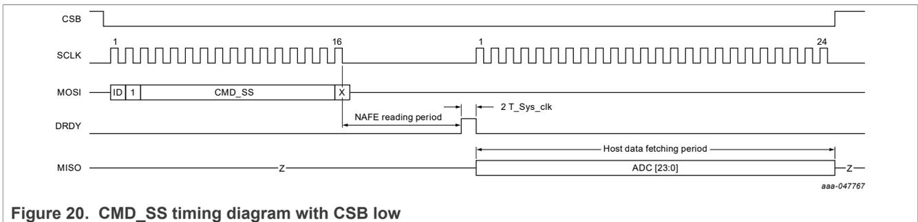
Figure 20. CMD\_SS timing diagram with CSB low
