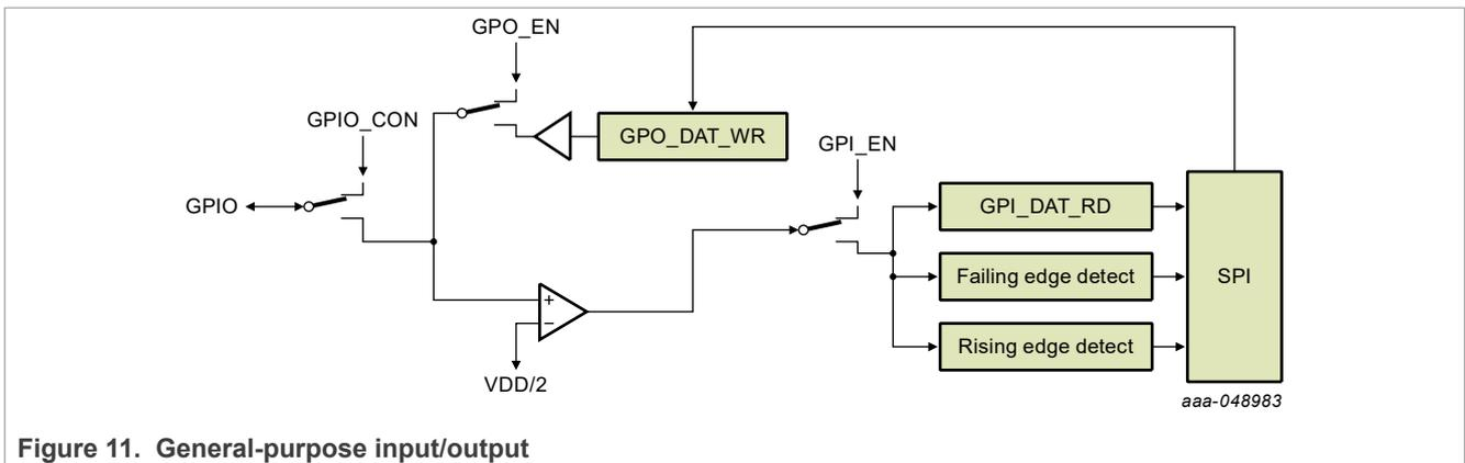
Figure 11. General-purpose input/output
