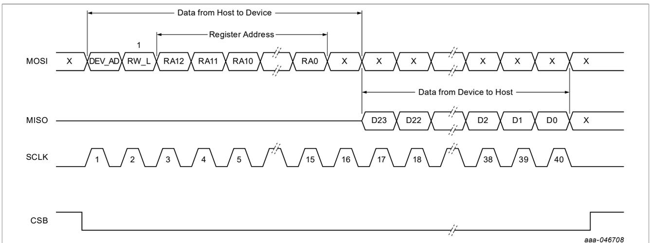
Figure 32. SPI read timing
