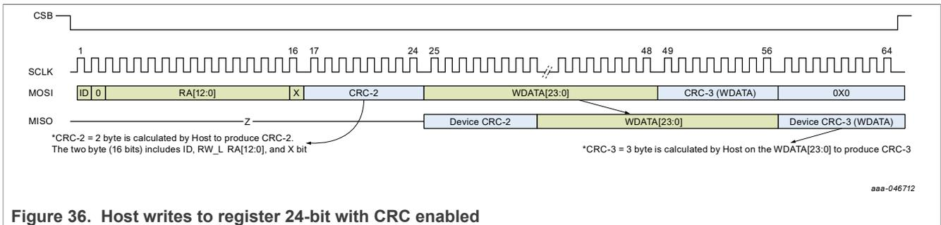
Figure 36. Host writes to register 24-bit with CRC enabled
