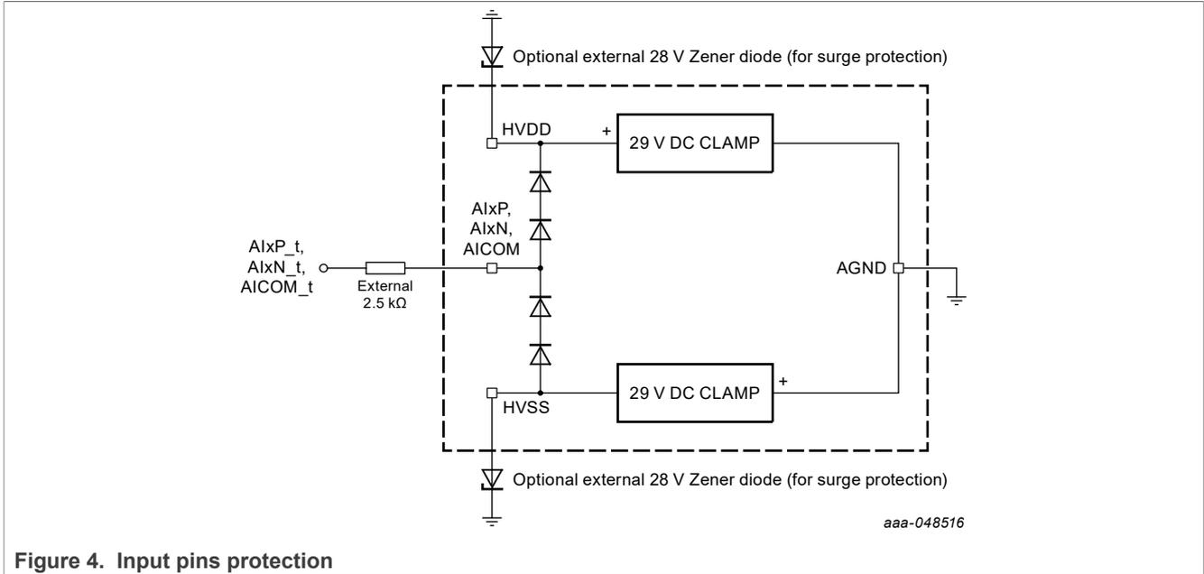
Figure 4. Input pins protection
