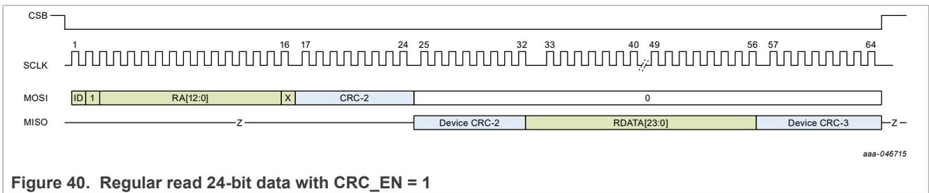
Figure 40. Regular read 24-bit data with CRC\_EN = 1
