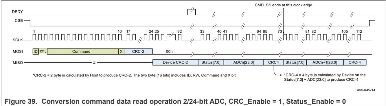
Figure 39. Conversion command data read operation 2/24-bit ADC, CRC\_Enable = 1, Status\_Enable = 0
