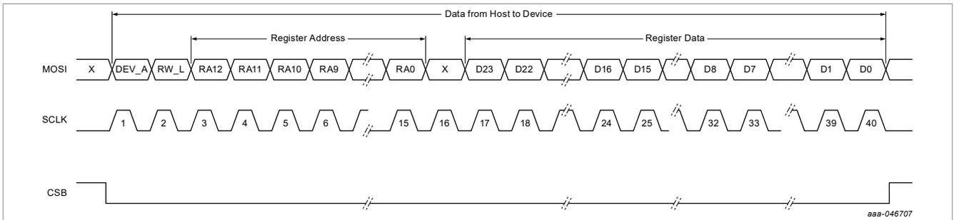
Figure 31. SPI write timing
