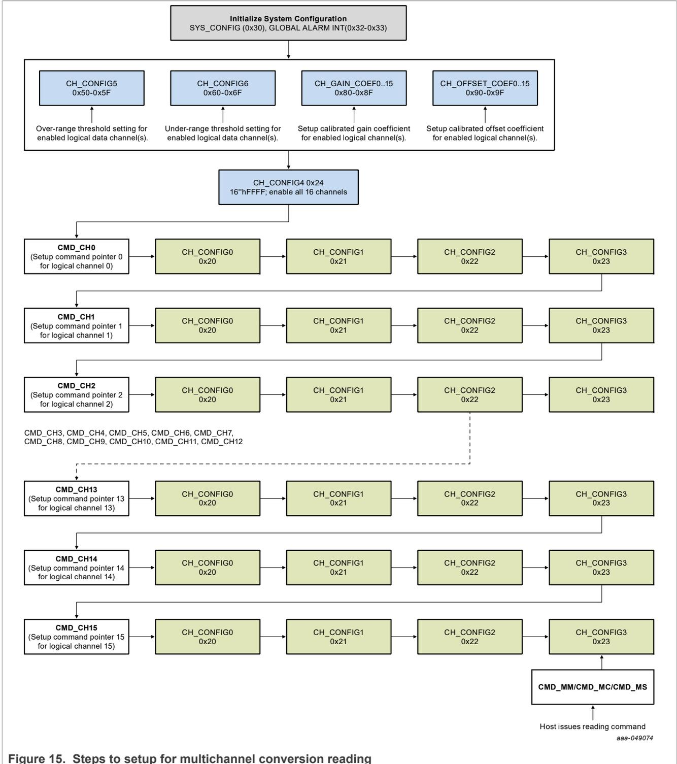
Figure 15. Steps to setup for multichannel conversion reading
