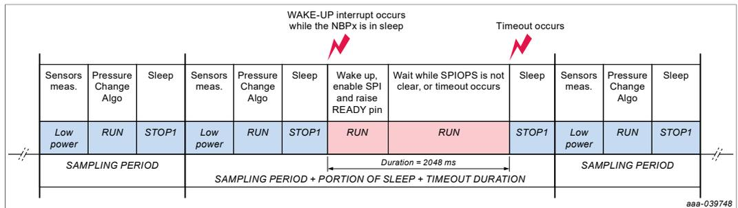
Figure 17. External host requests SPI transfers but does not clear the SPIOPS register
