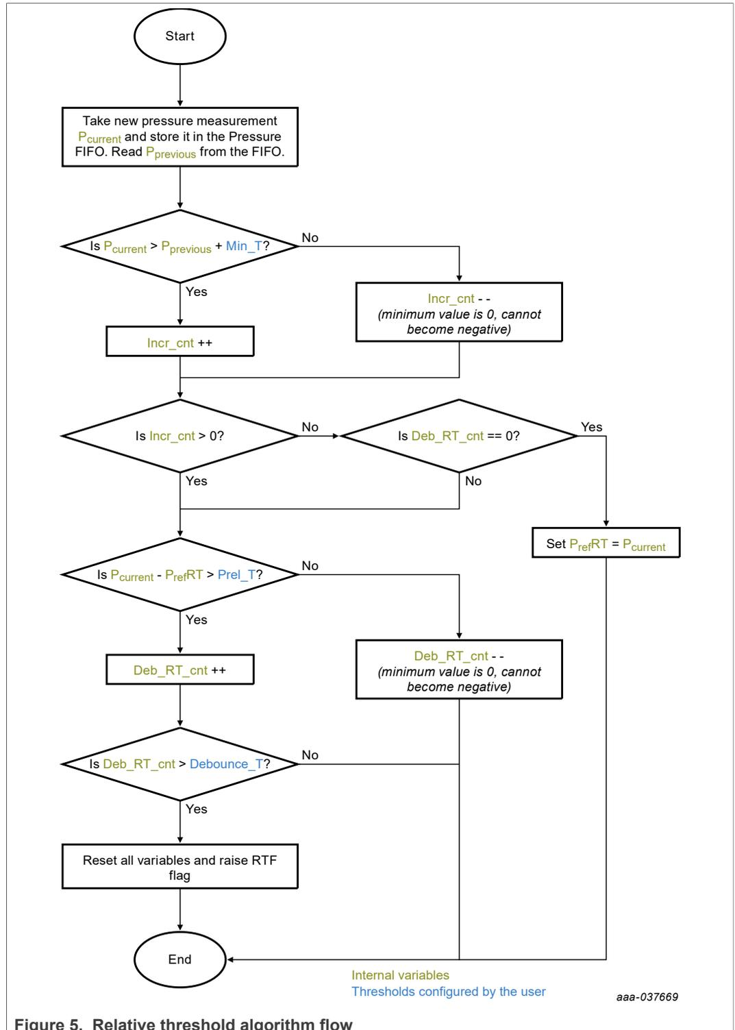
Figure 5. Relative threshold algorithm flow
