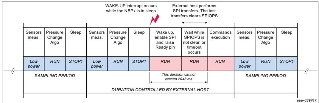
Figure 16. External host requests SPI transfers and then clears the SPIOPS register
