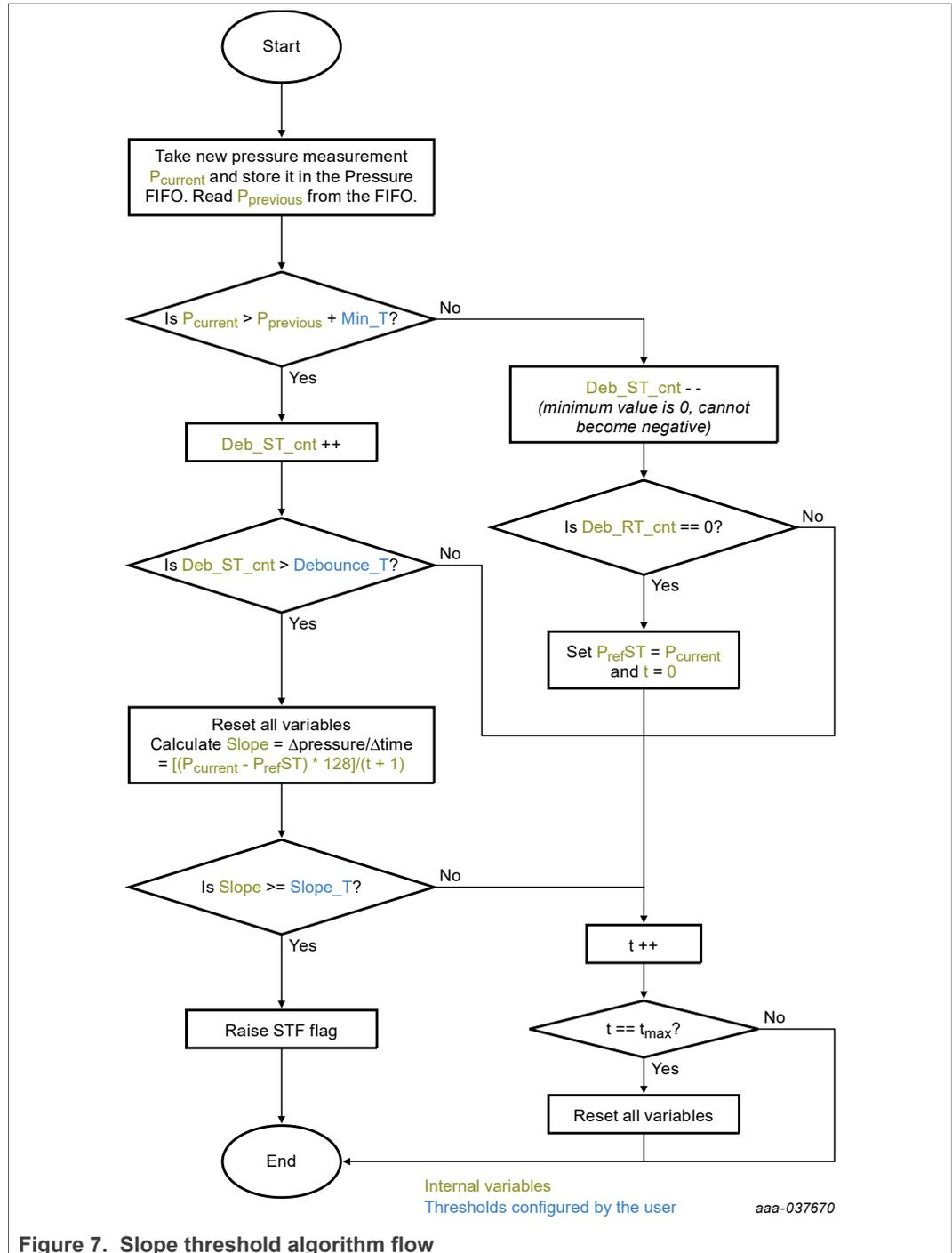
Figure 7. Slope threshold algorithm flow
