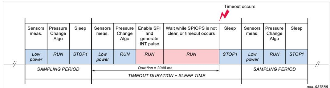
Figure 15. Sequence of events when NBPx notifies the external host of an event but the external host does not clear the SPIOPS register
