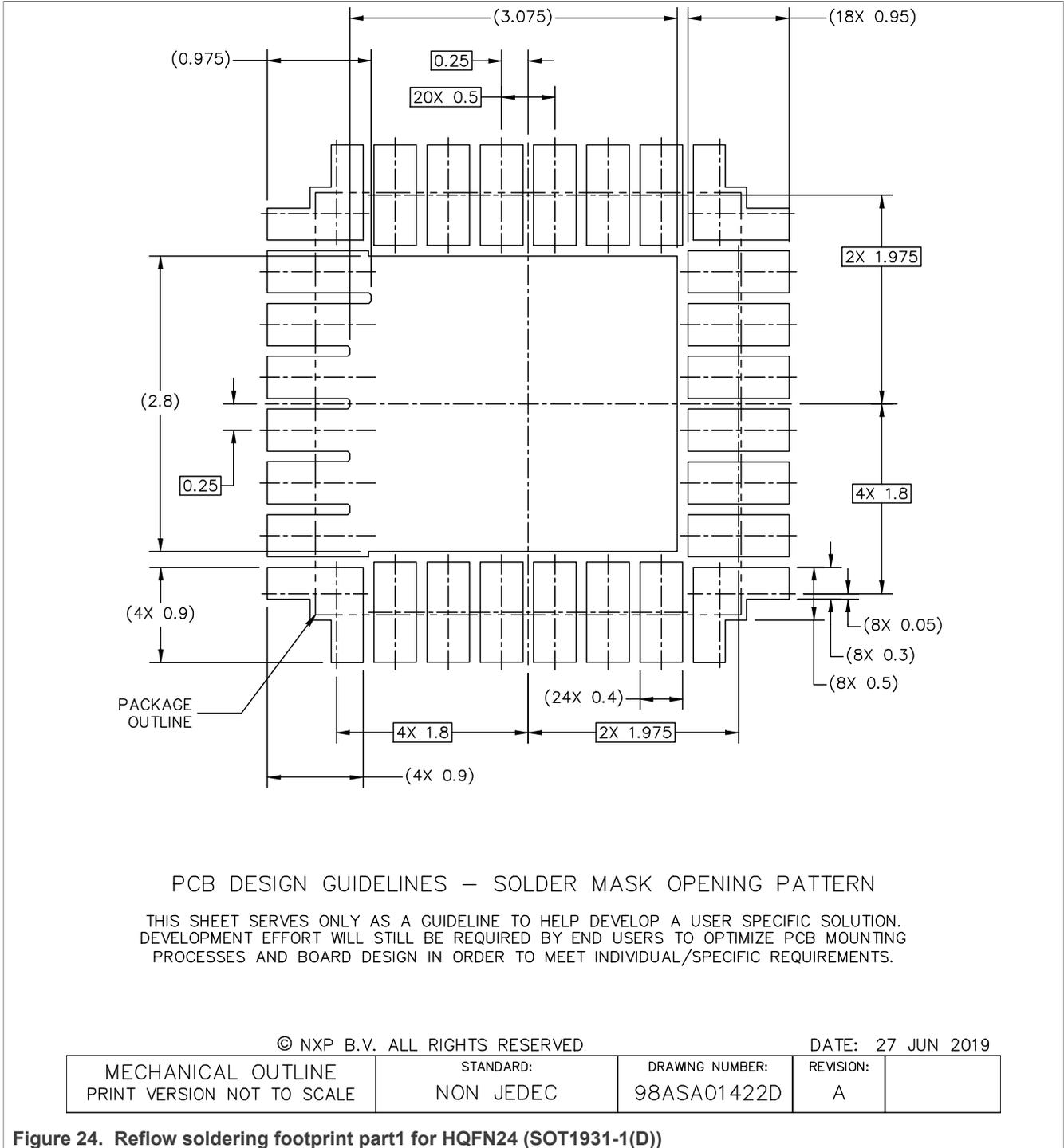
Figure 24. Reflow soldering footprint part1 for HQFN24 (SOT1931-1(D))
