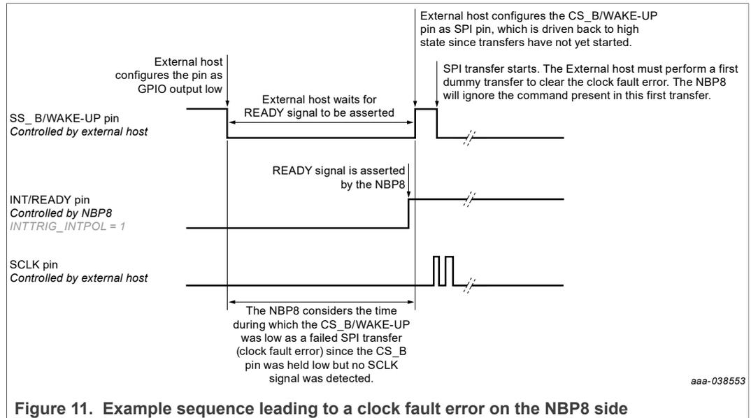
Figure 11. Example sequence leading to a clock fault error on the NBP8 side
