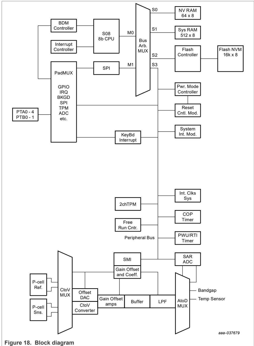
Figure 18. Block diagram
