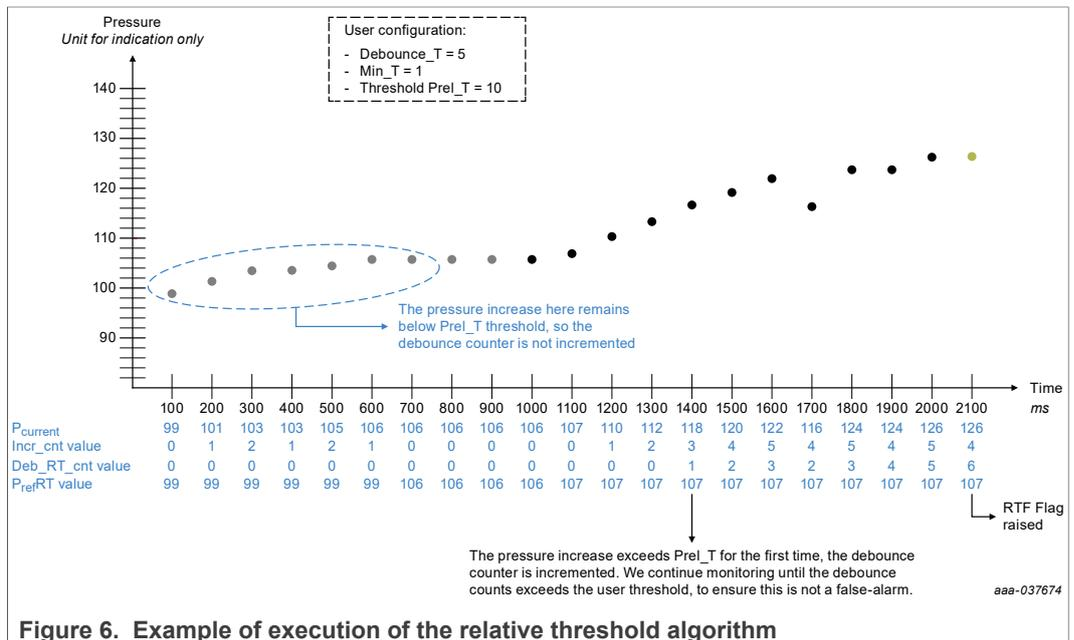
Figure 6. Example of execution of the relative threshold algorithm
