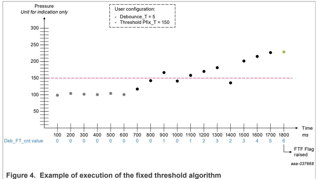
Figure 4. Example of execution of the fixed threshold algorithm
