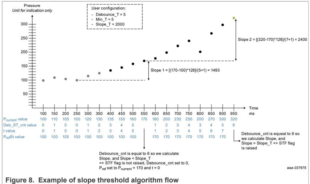
Figure 8. Example of slope threshold algorithm flow
