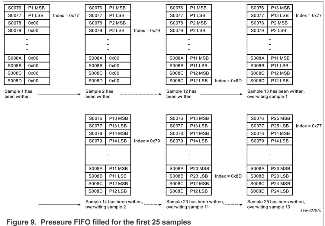
Figure 9. Pressure FIFO filled for the first 25 samples
