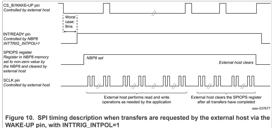
Important note: [Figure 10](#) shows that the CS\_B / WAKE-UP pin is held low by the external host from the moment the external host lowers the pin to request a transfer, until the end of the first SPI transfer. In reality, the actual sequence implemented by the external host may be different, taking into account the possible software implementation described below.
