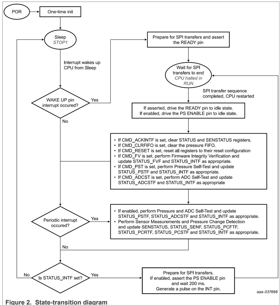
Figure 2. State-transition diagram
