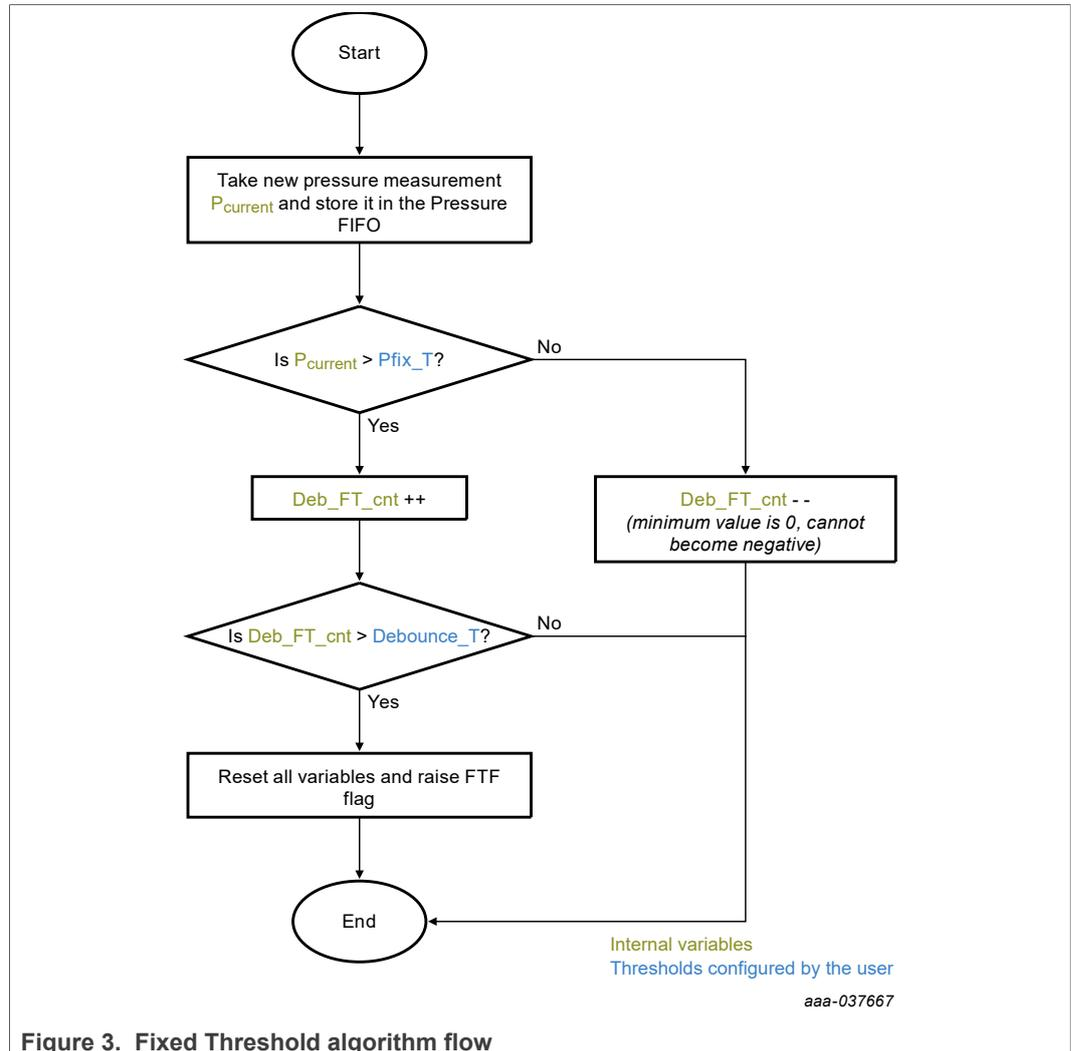
Figure 3. Fixed Threshold algorithm flow
