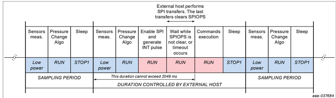
Figure 14. Sequence of events when NBPx notifies the external host of an event and the external host clears the SPIOPS register
