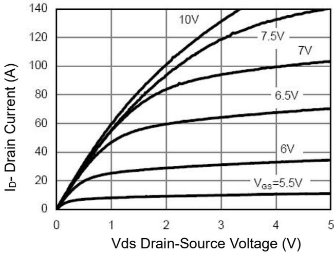
Figure 1 Output Characteristics
