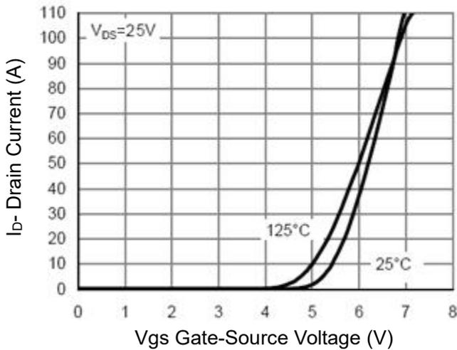
Figure 2 Transfer Characteristics
