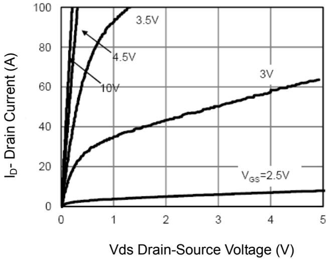
**Figure 1 Output Characteristics**
