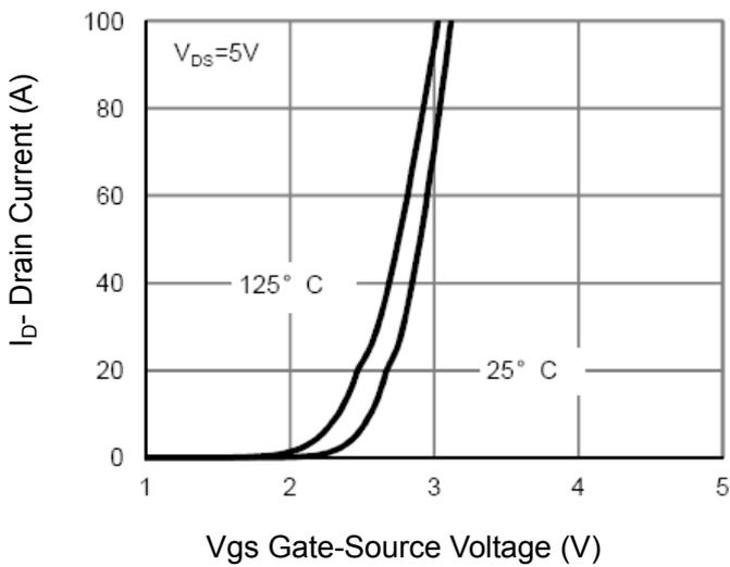
**Figure 2 Transfer Characteristics**
