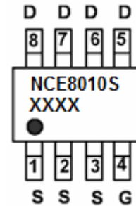
Marking and pin assignment
