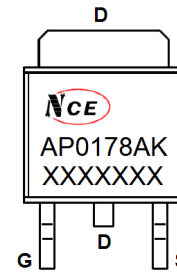
Marking and pin assignment
