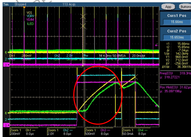
Figure 31. Minimum Dimming Duty Cycle
