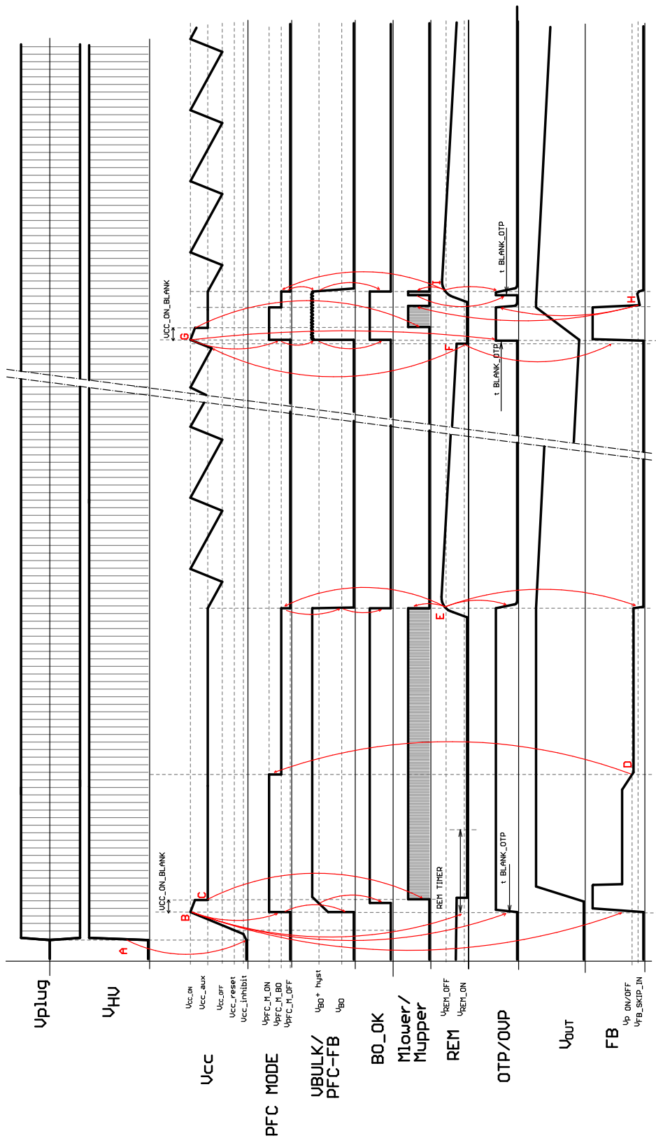
Figure 64. Start-up, Normal Operation, Transition to Off-mode Operation and Output Re-charge in Off-mode – NCP1399By Version
